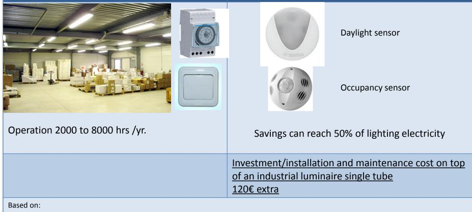
1.5 m , 35 W Single T5 no diimming 130 € , with dimming (0-10 v, DALI) : 250€ Typical savings per year 1500 hrs x 6 W/m2 = 9 Kwh/m2.yr →value 1,35€/m<sup>2</sup> Investment, per m2 : one luminaire per 10 m<sup>2</sup>: 12 €/m<sup>2</sup>
