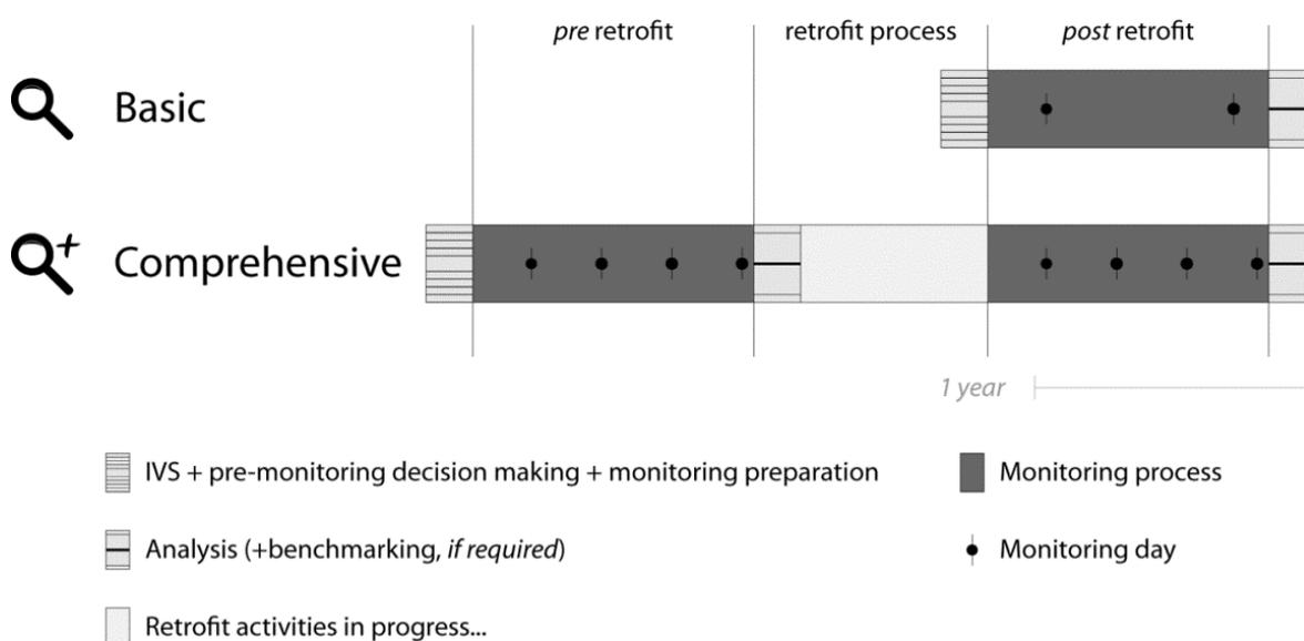
Figure 2 Schematic description of the general monitoring procedure.
