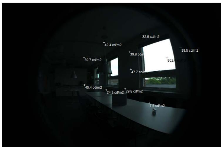
**Figure 10** Example of a HDR image produced using WebHDR and opened in the Radiance image viewer.
