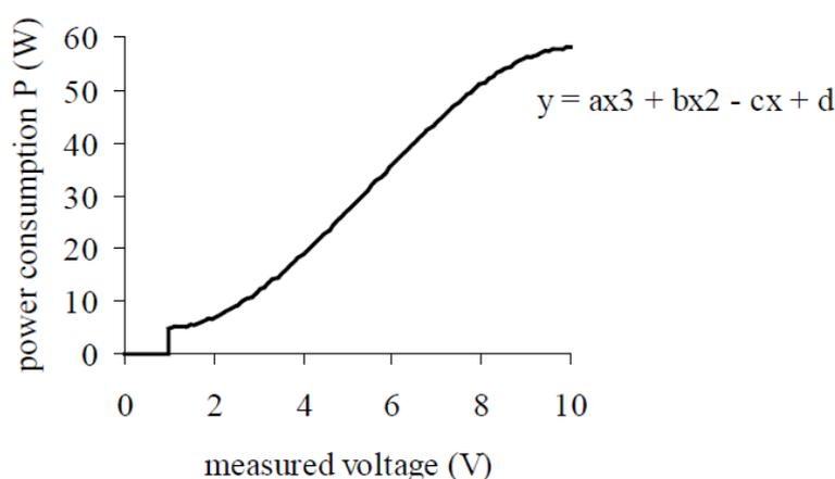
**Figure 8** Example of relation between measured voltage and the power consumption of electric lighting, from Velds & Christoffersen (2001).
