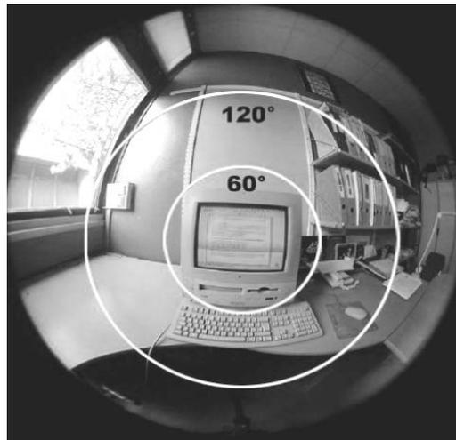
**Figure 4** Picture showing the ergorama ( $60^\circ$ ) and panorama ( $120^\circ$ ), according to Sutter, Dumortier, & Fontoynt (2006).
