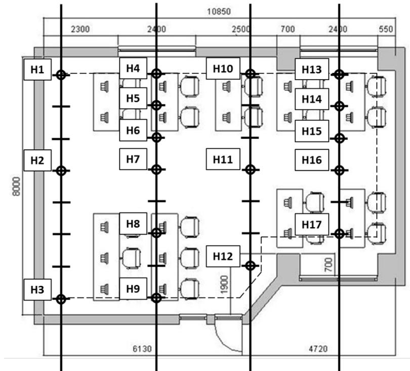
Figure 7 Possible position of sensors in an irregularly shaped room.
