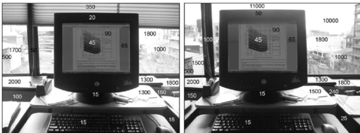
**Figure 5** Example of photographs of a task with superposed luminance spot measurements, by Madsen & Osterhaus (2014).
