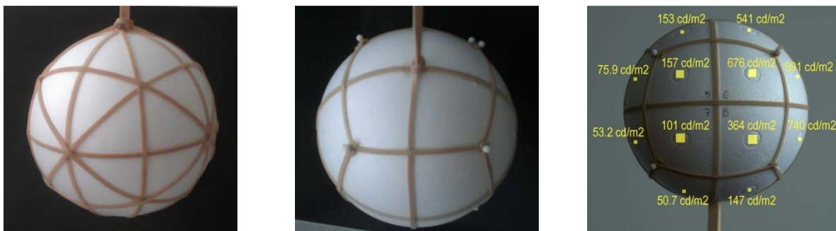
**Figure 11** Diffuse white sphere with surface divided into 24 similar areas using elastic bands and pins and luminance values retrieved from the HDR image of the sphere.
